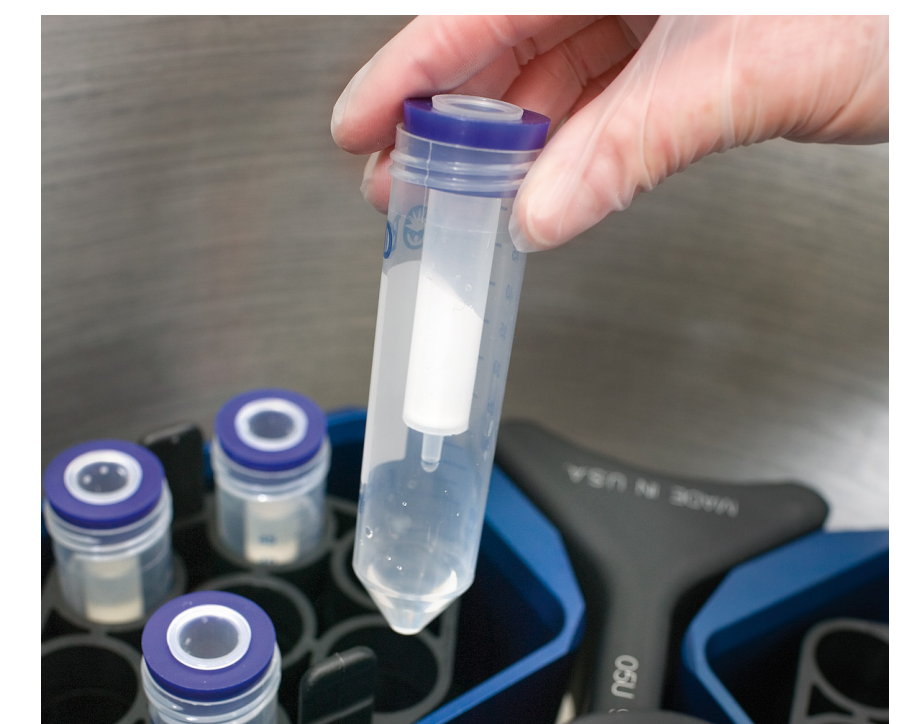
Fig 5.14. Spin adapters enable the use of PD-10 Desalting column, as well as PD MidiTrap G-25 and PD MiniTrap G-25 columns in a standard centrifuge.
